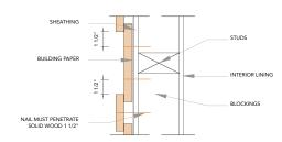
Face nail through center of batten and double nail siding.
